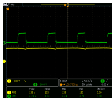
Figure 15. Gate Pulse of MOSFET at 120 V AC source
