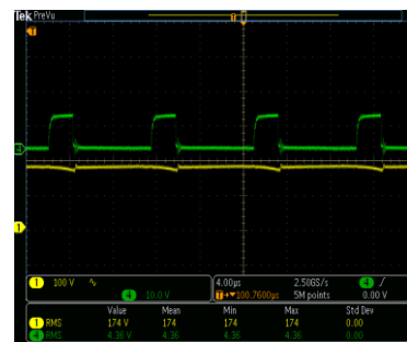
Figure 16. Gate Pulse of MOSFET 230 V AC source
