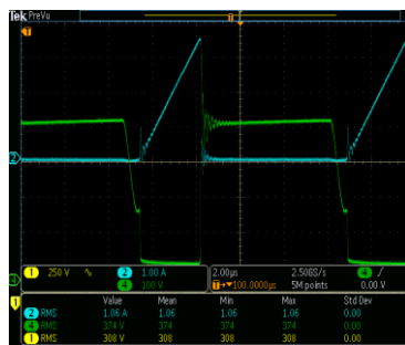
Figure 14. Drain- Source voltage and drain current at 230 V AC
