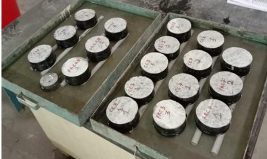
Figure 7 Sorptivity test configuration
