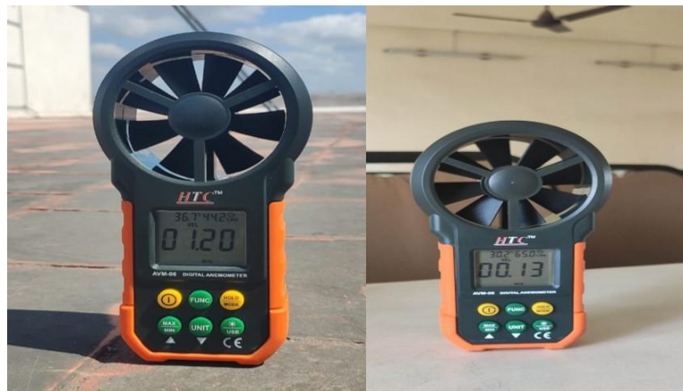
Figure: 11 Shows the Anemometer HTC AVM-06
