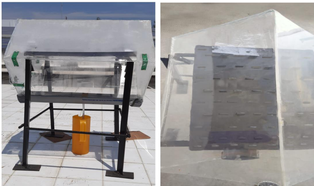
Figure 3. Experimental setup of triangular solar still with fins.
