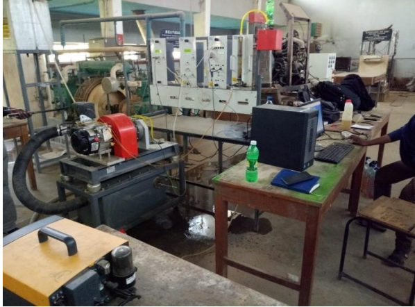
Figure 1. Experimental setup for the performance and emission test analyser setup
