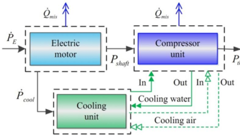
Fig. 4. Energy balance of searable compressor driven by electric motor
