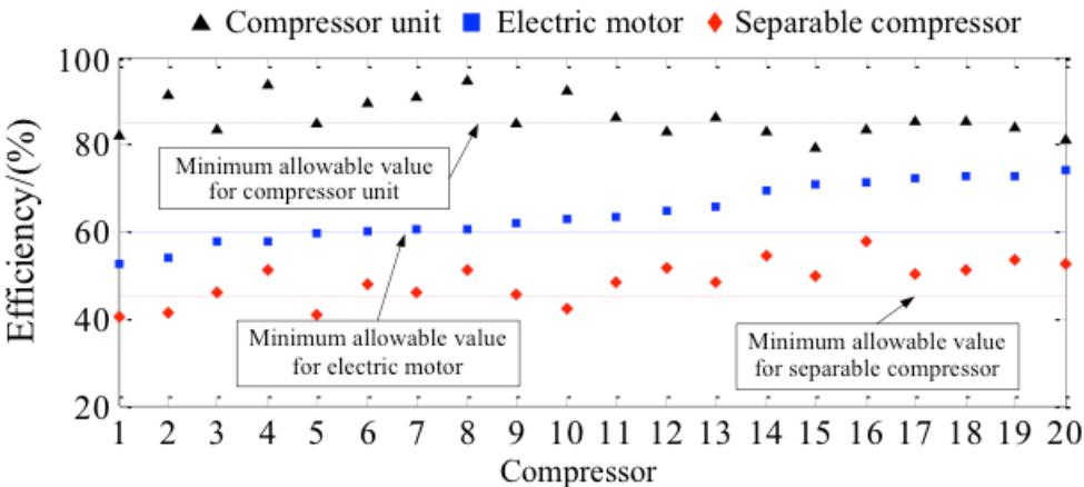
Fig. 11. Various kinds of efficiencies of separable compressors
