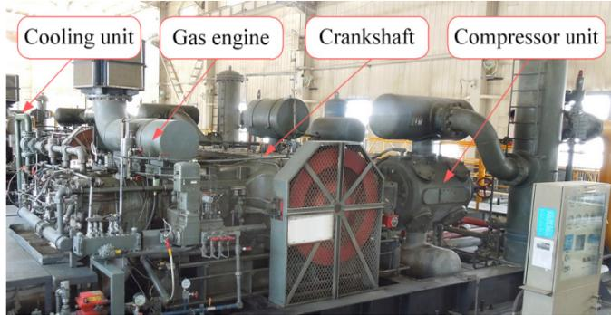
Fig. 1. Integral engine compressor driven by gas engine
