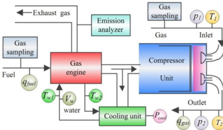
**Fig. 5.** Experimental setup of integral engine compressor
