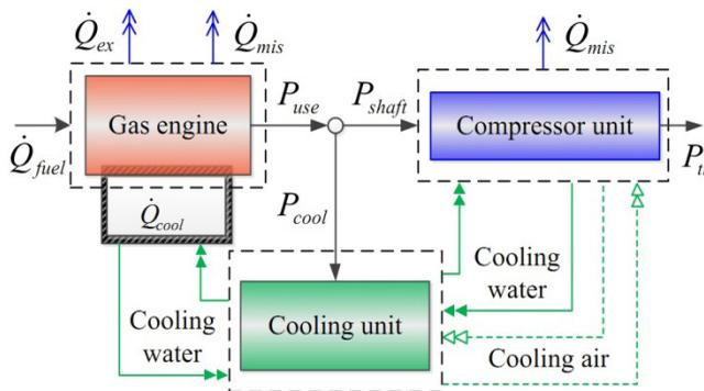
Fig. 2. Energy balance of integral engine compressor
