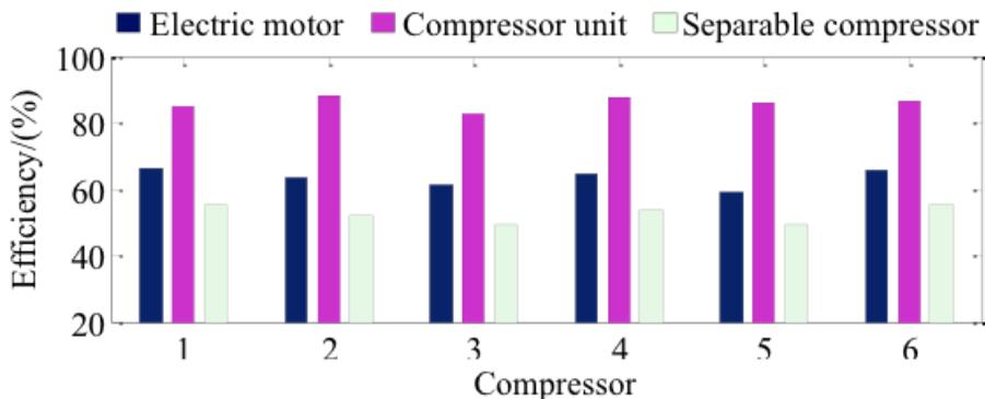
**Fig. 9.** Results of separable compressor efficiencies
