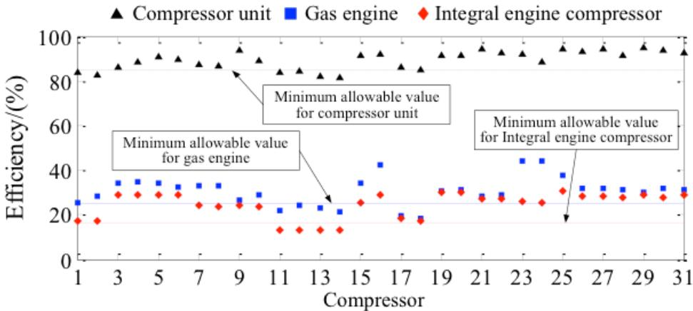
Fig. 10. Various kinds of efficiencies of integral engine compressors
