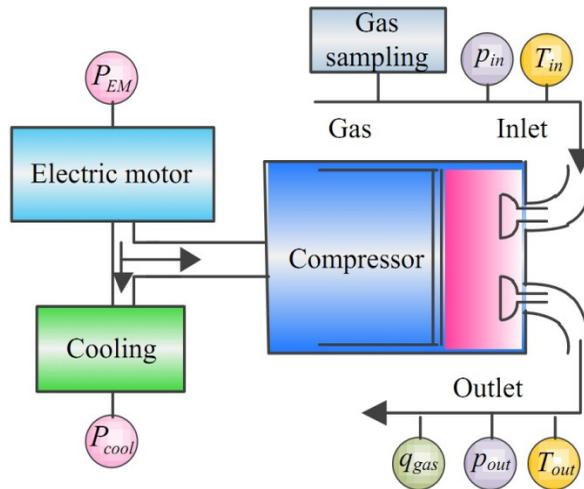
Fig. 8. Experimental setup of separable compressor
