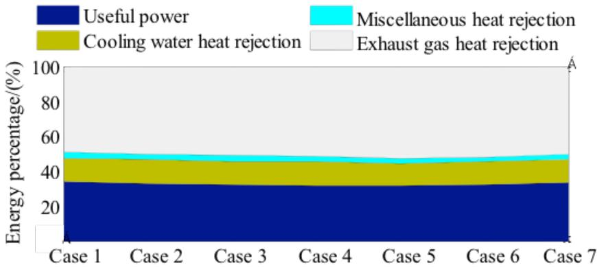
Fig. 7. Energy distribution of integral engine compressor
