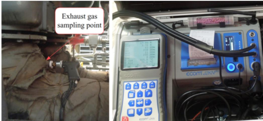
**Fig. 6.** Exhaust gas composition test on integral engine compressor
