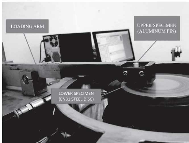
Figure 2. Tribometer in working condition.
