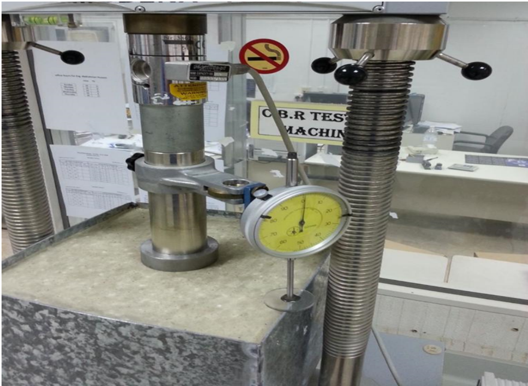
Figure 6a. Load test set up on clayey sand (gatch) soil.
