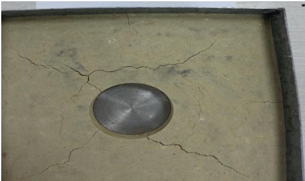
Figure 6b. After failure view showing punching failure and radial cracks (RC = 90%).
