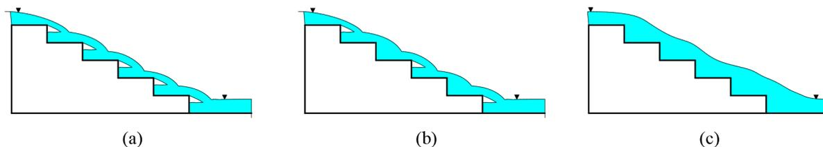
**Figure 1** Flow regimes on the stepped spillway: a) nap flow regime; b) transition flow regime; c) skimming flow regime (Takahashi et al. 2001)
