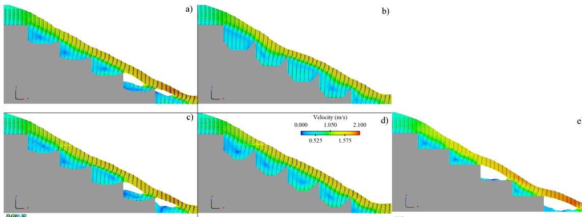
**Figure 9** Velocity vectors of models: a) Model 1, b) Model 2, c) Model 3, d) Model 4, and e) Classical stepped
