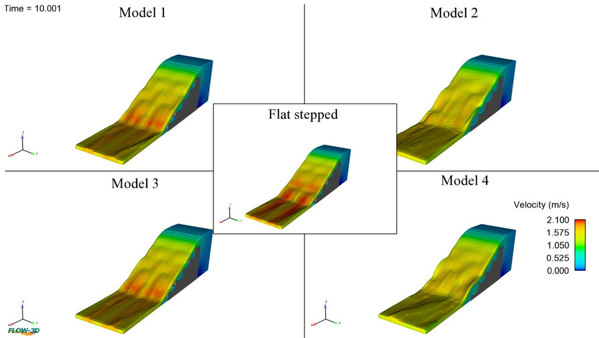
**Figure 8** Three-dimensional velocity profiles for skimming flow regime
