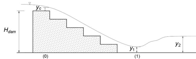
**Figure 4** Longitudinal section of spillway
