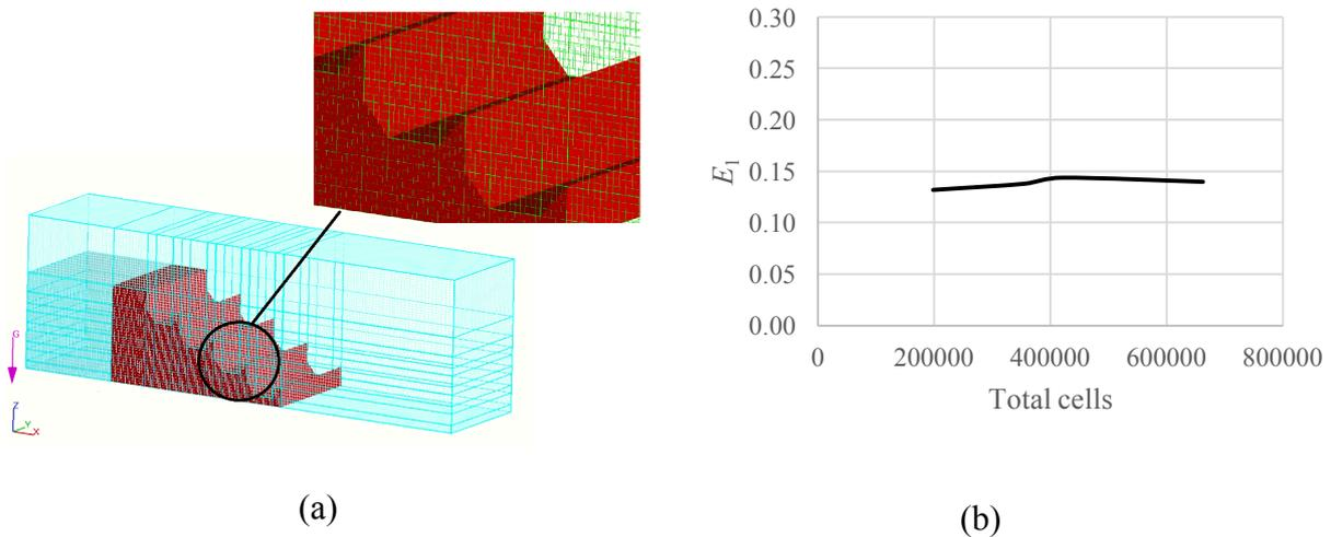
Figure 5 a) Mesh domain structure and b) Mesh independency
