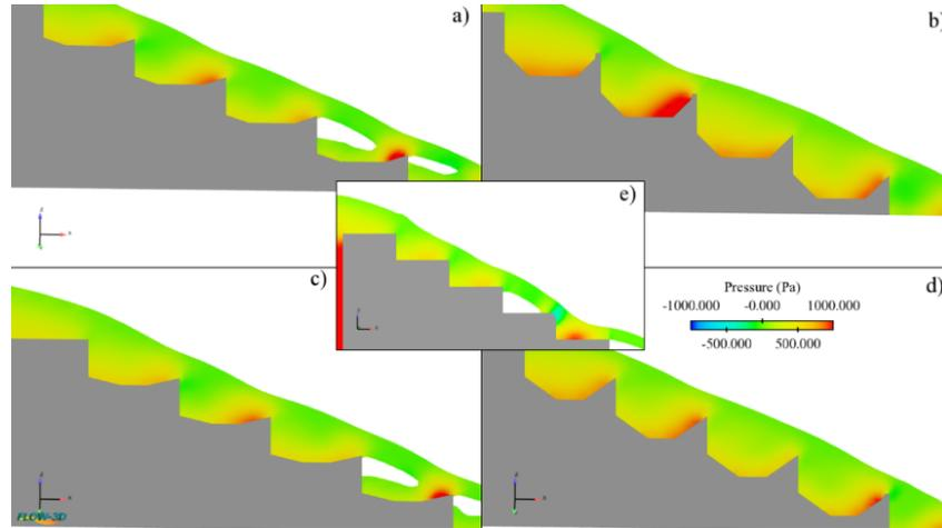
**Figure 10** Pressure contours of models: a) Model 1, b) Model 2, c) Model 3, d) Model 4, and e) Classical stepped
