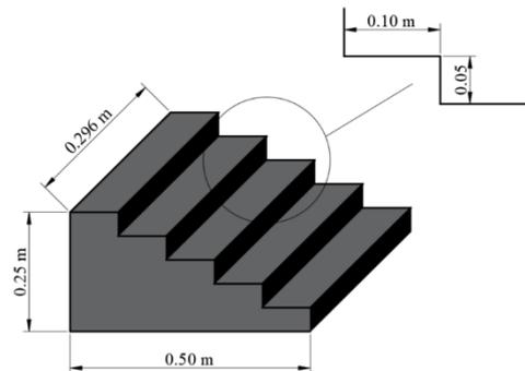
**Figure 2** The model geometry designed by Mero and Mitchell (2017)
