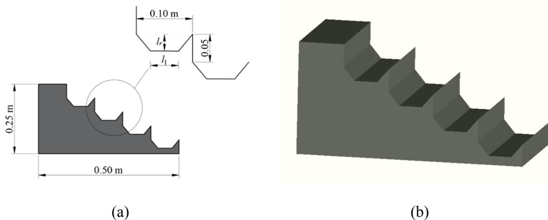
**Figure 3** The design of the TSS; a) two-dimensional, b) three-dimensional
