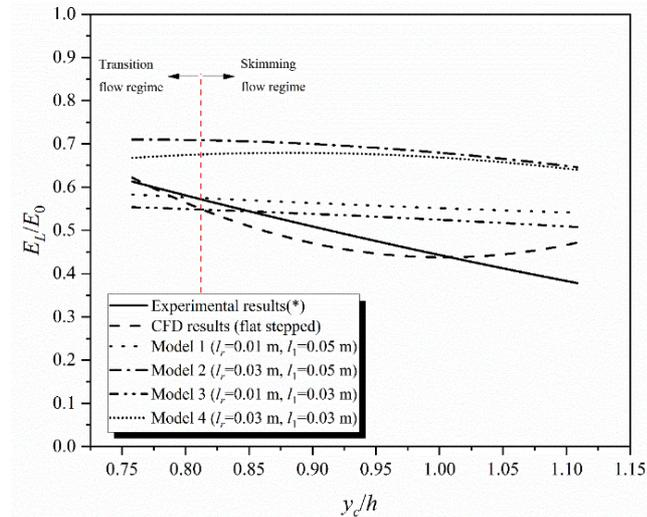
**Figure 13** Comparison of the energy dissipation rate of the used models
