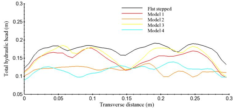
**Figure 12.** The total hydraulic head of the models on the transverse section
