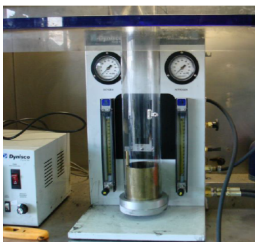
Figure 2. Limiting oxygen index chamber
