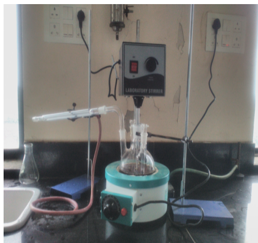
Figure 1. Transesterification process setup sketch and actual photograph
