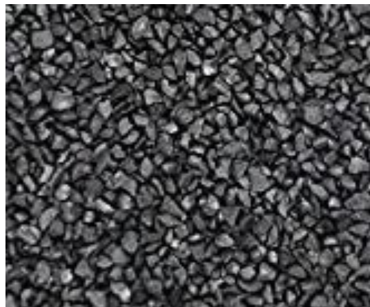
Figure 1. Steel grit G25 particle (particle size: 0.71– 1.19 mm).
